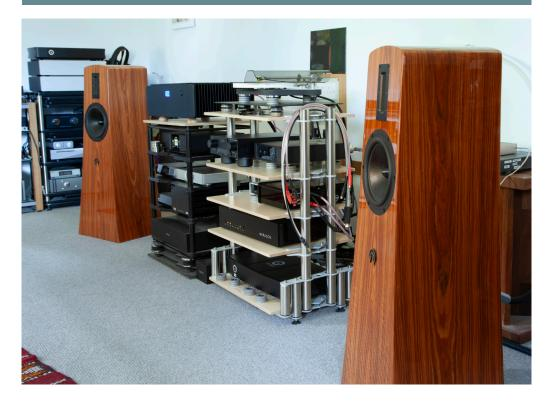
combined with the unusual bass loading system, made it hard to find the optimal position for the Altas. In the end they were widely spaced (2.4m) and angled so that they fired directly at the listening position with a gap of 70cm to the rear wall - further into the room than average in this space but not excessive.
