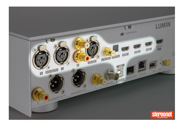
Something I haven't seen previously on network streamers is the provision for a fibre-optic networking connection as well as the regular RJ45 Ethernet socket. There is a slot that accepts an aftermarket SFP module, which stands for small form-factor pluggable. It is an optical transceiver module typically used in data communication networks. Being an optical connection, it is galvanically isolated, so immune to digital network noise
