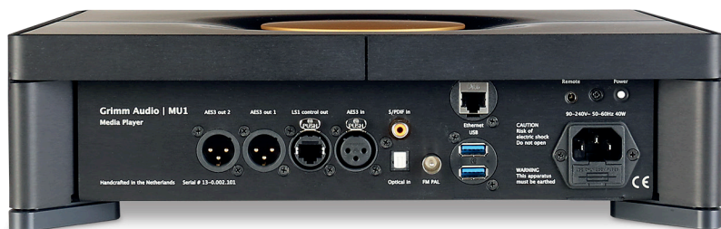
ABOVE: Digital only, as the MU1 offers a network control/streaming input, coax/optical S/PDIF and AES inputs. USB-As cater for storage and DAC connections, with dig outs on single/dual-AES XLRs and a proprietary RJ45 link for Grimm's LS1 loudspeaker
