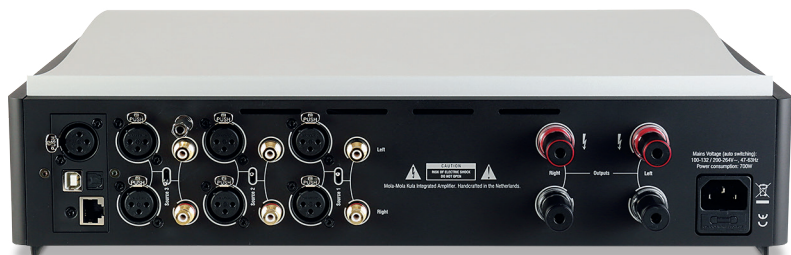
ABOVE: Three analogue ins on RCAs and XLRs (switched) are routed via optional phono or line stages. Digital module [far left] includes Toslink optical and AES/EBU (to 192kHz/24-bit) plus USB-B and Ethernet (384kHz/32-bit and DSD512). The speaker outputs are on Furutech 4mm terminals wired internally with Kubala-Sosna cable
