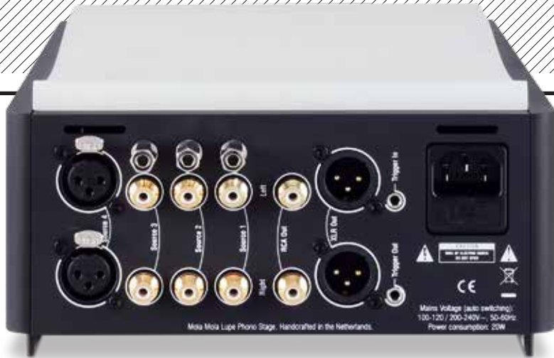
ABOVE: The three RCA inputs and one XLR (the latter only truly balanced with MCs) may be routed to entirely separate MM and MC phono amplifiers within. Outputs are directed via the app [see p69] through the RCA and/or XLR terminals
